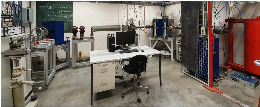
Figure 2: The new 100 kV Tandem accelerator at the mass separator for optimization of negative ion sources.
